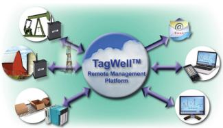
SoftPLC Gateways can provide access to other control systems via SoftPLC's TagWell Cloud Remote Management Platform (cell/satellite/etc) and via direct modem connections. The Gateway acts as a remote router access switch and/or as a data concentrator.
