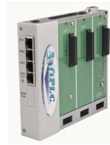
Smart SoftPLC w/ Backplane3 Interface (without and with modules installed)
